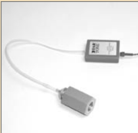
Figure A: Insert earphone attached to coupler
