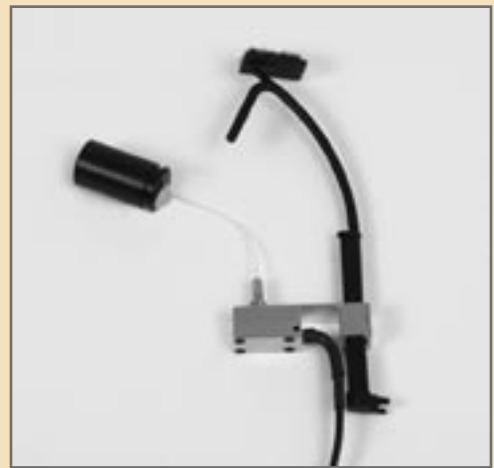
Figure B: Probe tube in probe mic adapter
