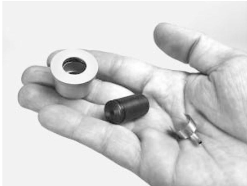
**Figure 4.1 Adapter, Probe Microphone Adapter, and Calibration Clip**
