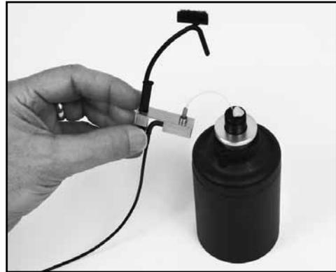
*Figure C-3: Integrated probe microphone inserted into sound calibrator.*
