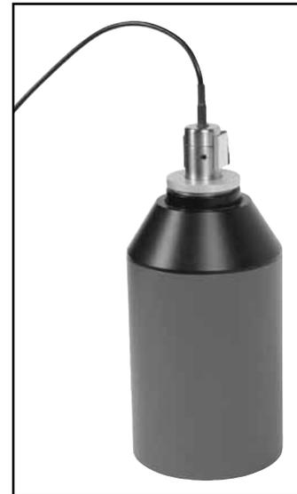
Figure C-2: Coupler microphone inserted into sound calibrator.
