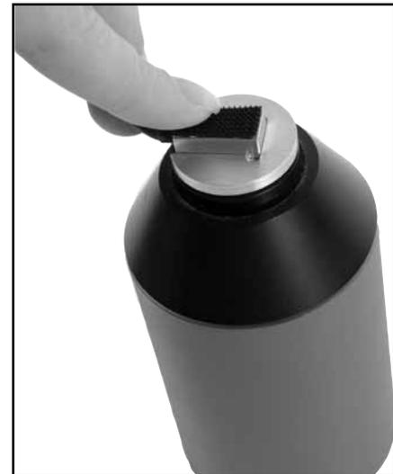
*Figure C-4: Rectangular reference microphone inserted into sound calibrator.*
