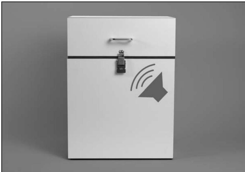
Figure 1—Sound chamber with speaker mount
