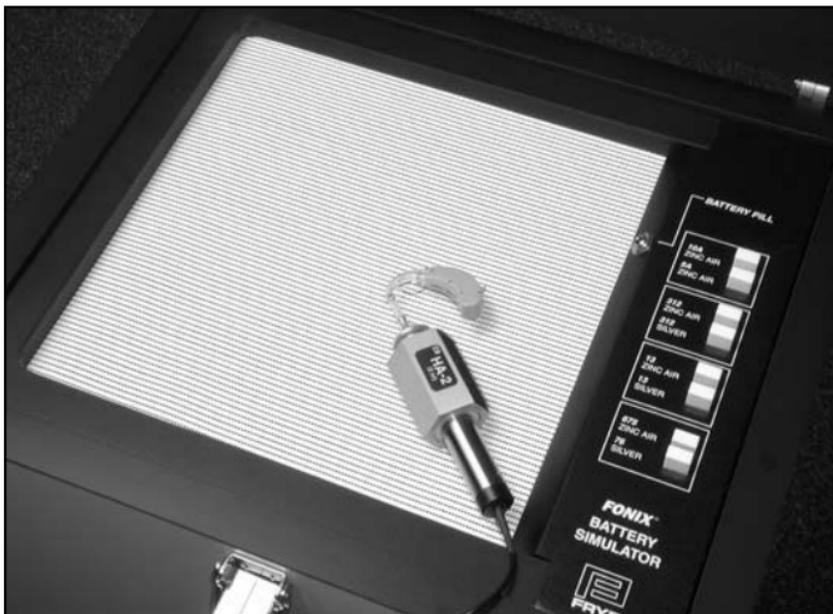
Figure 3—Reverse measurement in 7020 sound chamber
