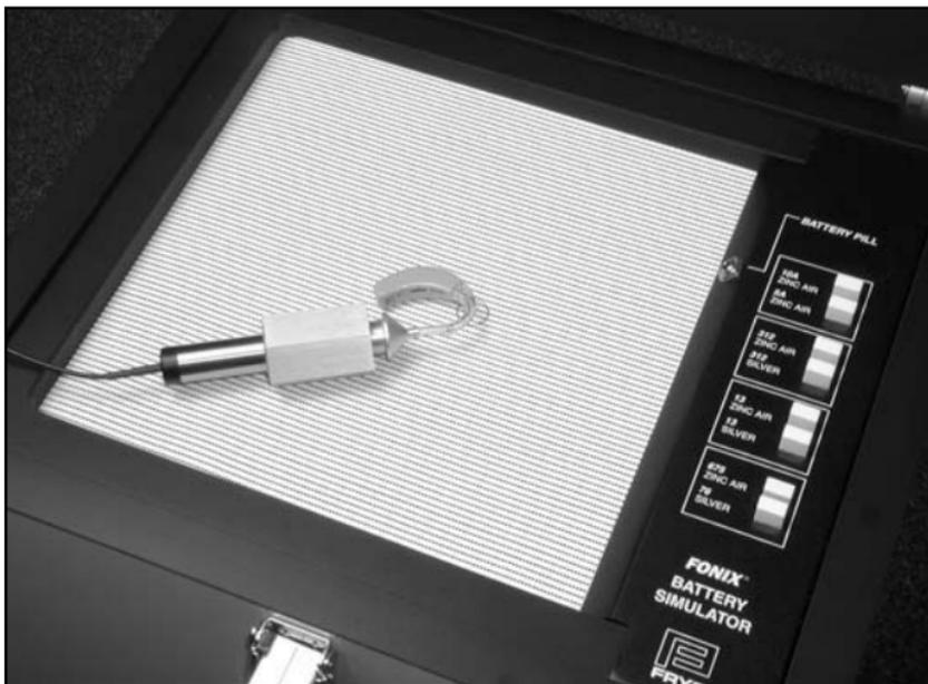
Figure 2—Forward positioning in 7020 sound chamber
