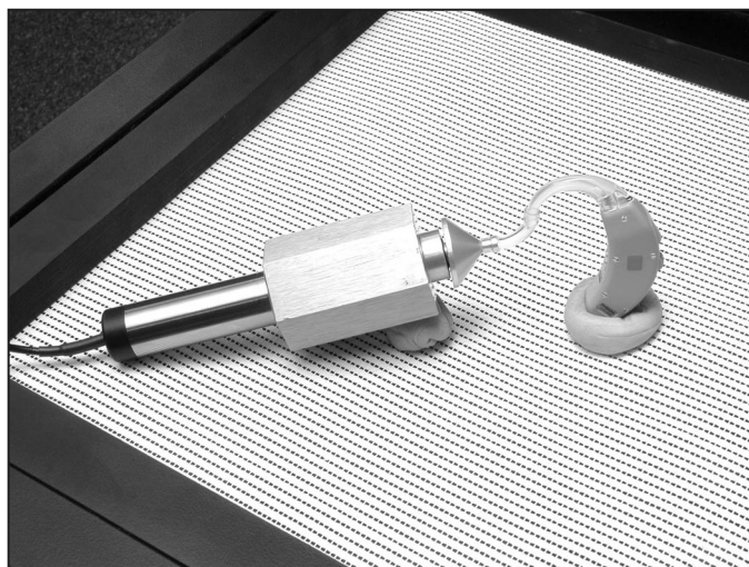
Figure 3.4.10A—Testing with the Sound Chamber Telecoil Board
