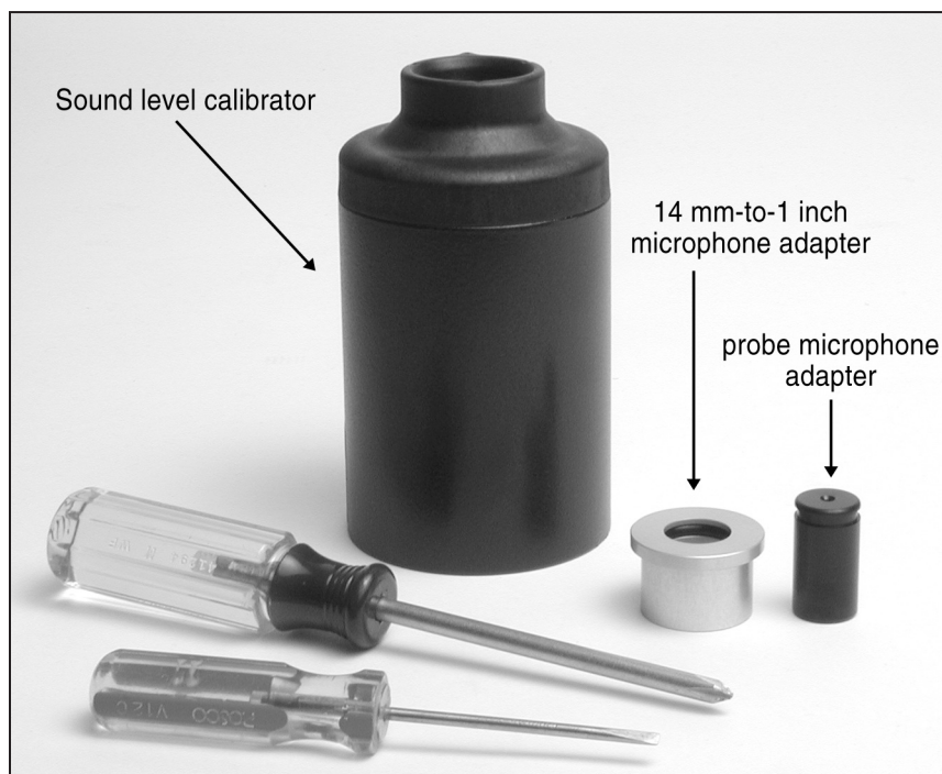
Figure B.1A—Equipment for calibrating the 7000 microphones.
