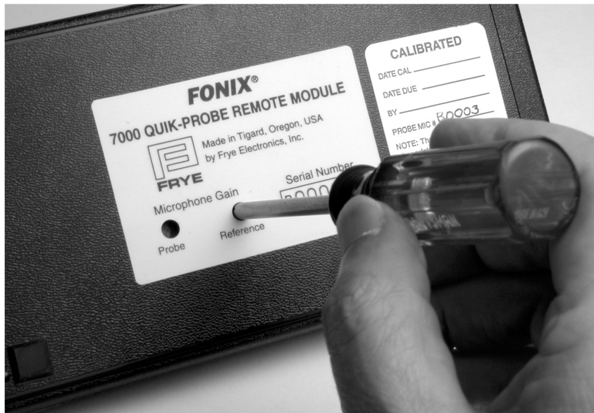
Figure B.1.C—Adjusting the reference pot with a Phillips-head screwdriver.
