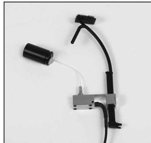
Figure 6.3.5B Probe tube in probe mic adapter
