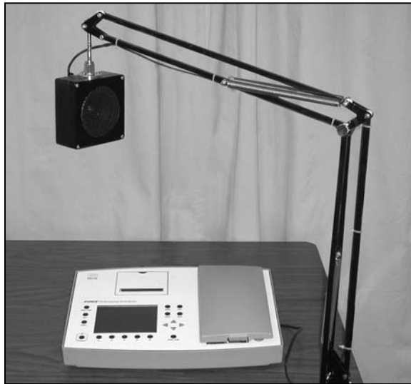
Figure 4.2.3—External sound field speaker setup
