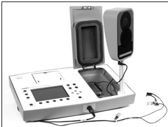
Figure 4.2.2—Internal sound field speaker setup
