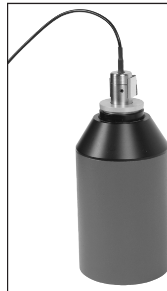
Figure 5.1.1: Coupler microphone inserted into sound calibrator.
