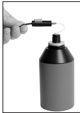
Figure 5.1.2B: Old-style probe microphone inserted into sound calibrator.
