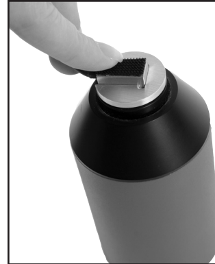
Figure 5.1.3: Rectangular reference microphone inserted into sound calibrator.
