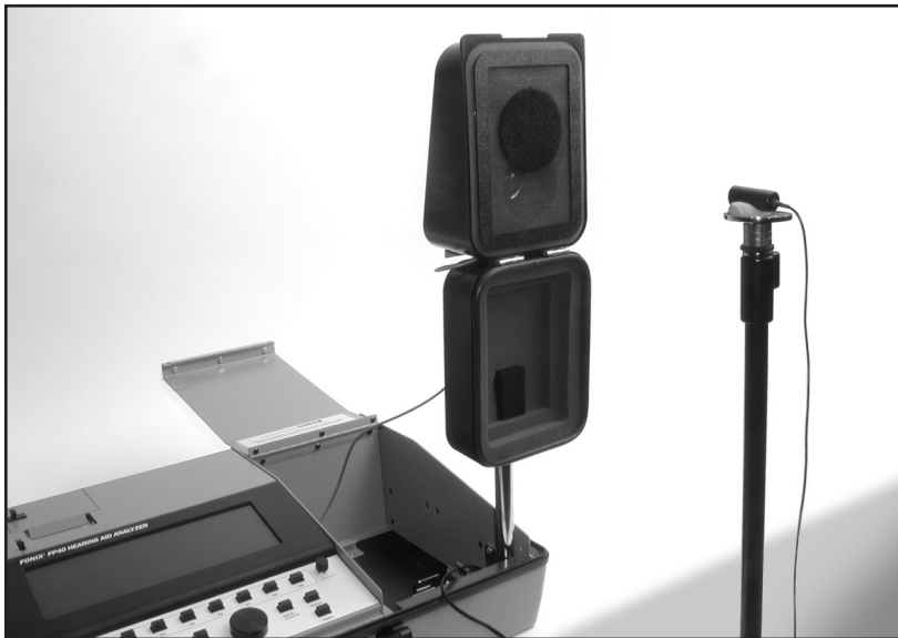
Figure 3.6.1—Preparing for a coupler directional measurement
