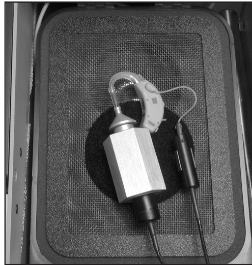
Figure 3.2.2—Leveling with reference microphone
