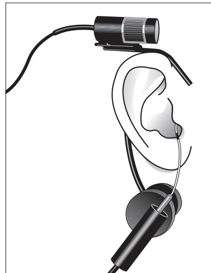
Figure 5.1.2.2—Placing the reference microphone
