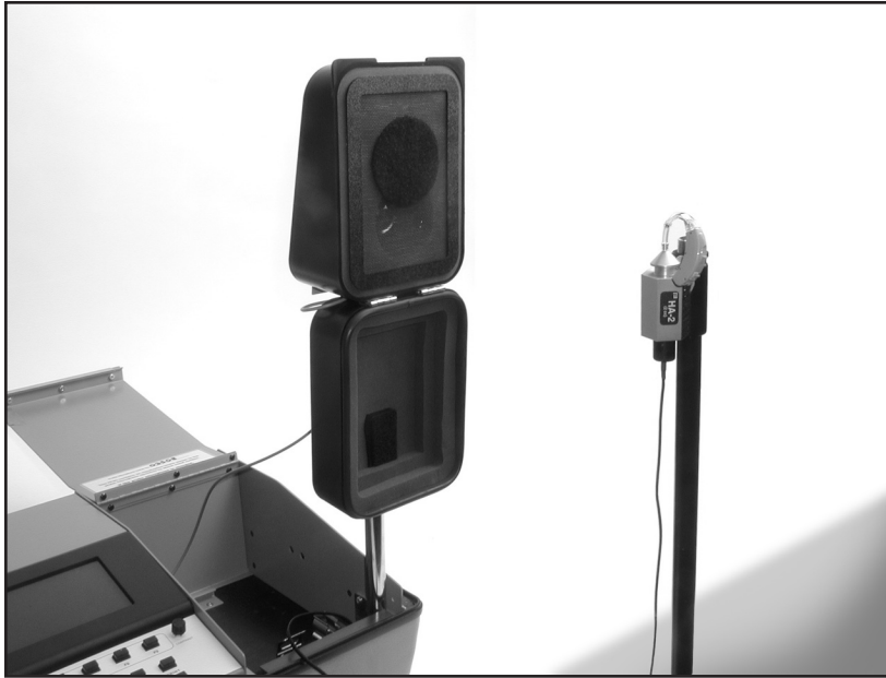
Figure 3.6.2—Testing the forward coupler response of a directional aid
