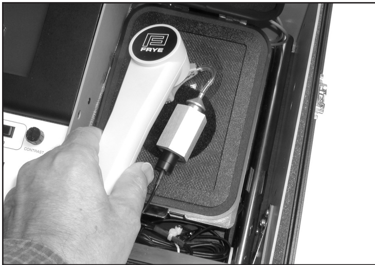
Figure 7.2 –Using the Telewand
