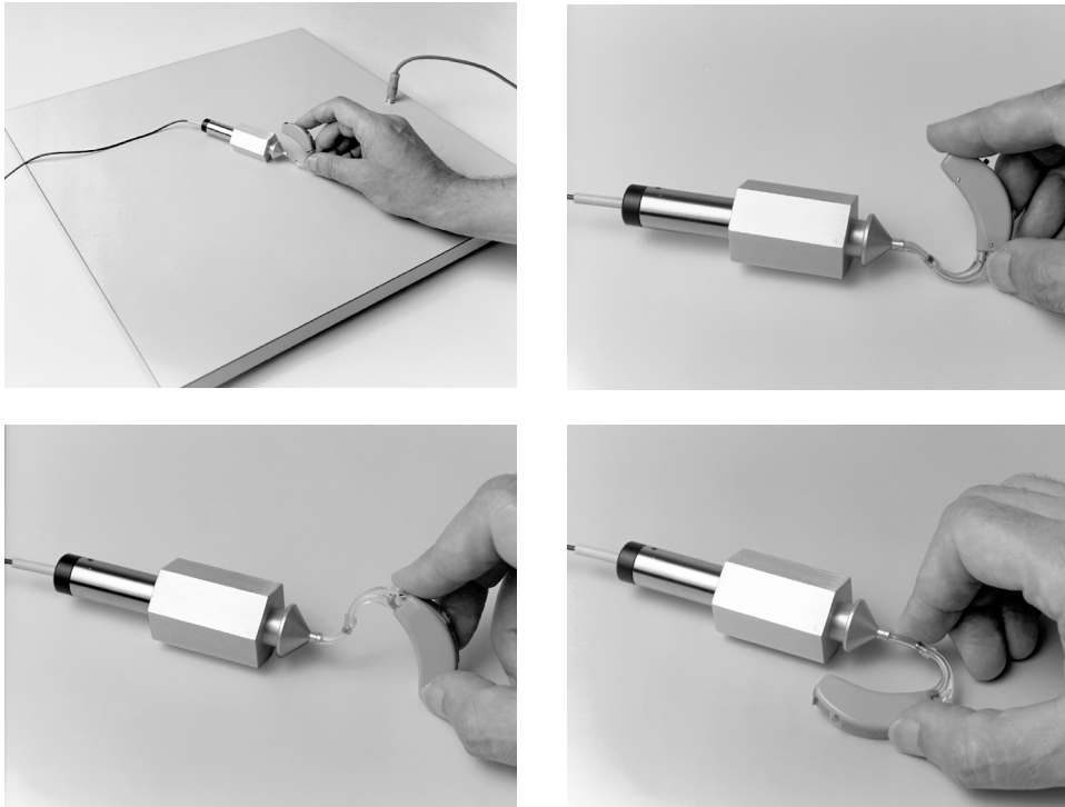
Figure 7.1B Orienting hearing aid for maximum output
