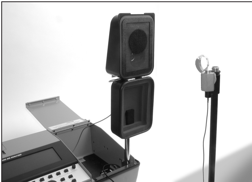
Figure 3.6.3 —Testing the reverse coupler response of a directional aid
