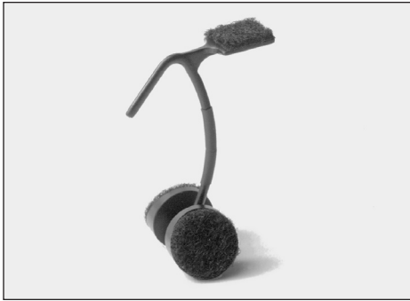
Child Size Wedge Style Earhook Holds probe and reference microphones during real ear testing.
