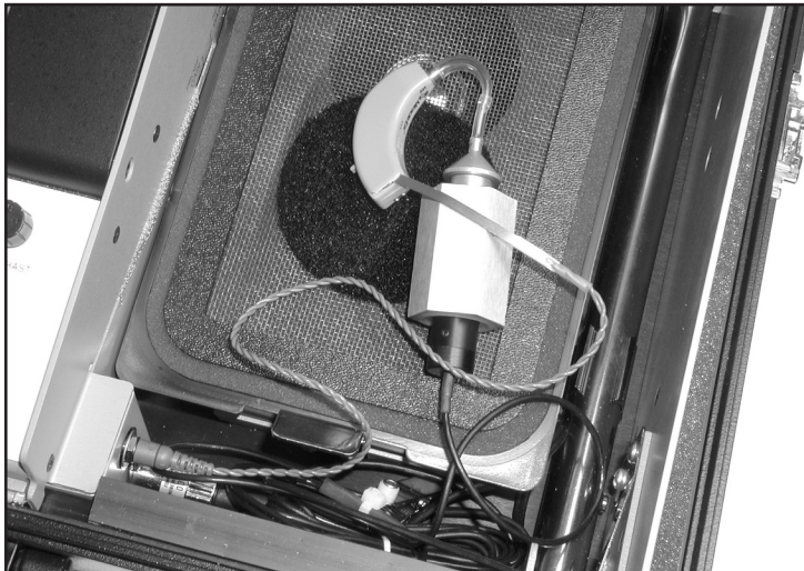
Figure 2.6A—Using a battery pill to measure the battery current drain
