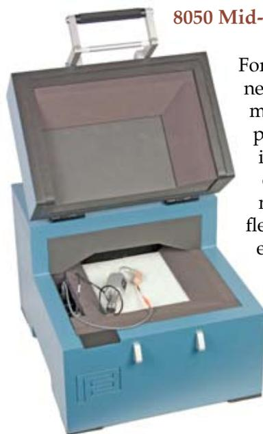
For those users who don't need to perform polar plot measurements, the compact 8050 sound chamber is available. This newly-designed chamber minimizes internal sound reflections while occluding exterior noise.
