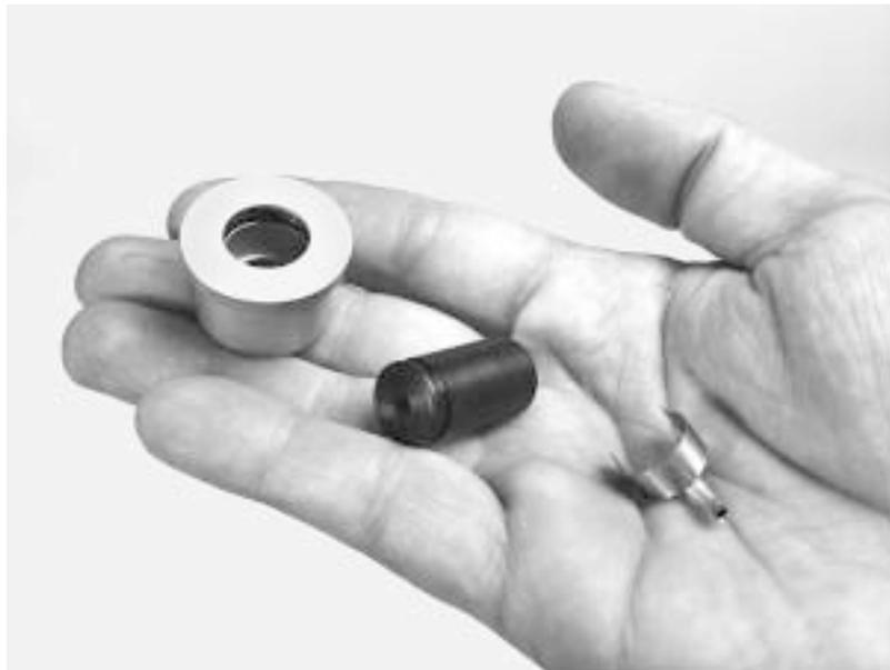
**Figure 8.6.1-1 —1" Adapter, 14-mm Probe Calibration Adapter, and Calibration Clip**
