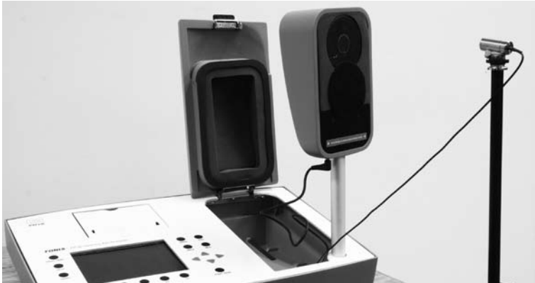
Figure 1: Leveling for coupler measurements using a sound field speaker
