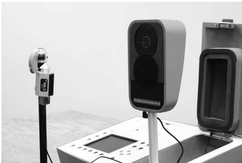
Figure 2: Performing coupler measurements using a sound field speaker
