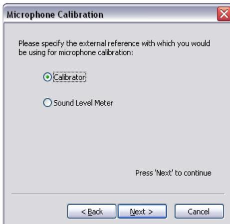
If you are performing the calibration process with a sound level calibrator (recommended), select **Calibrator**.
