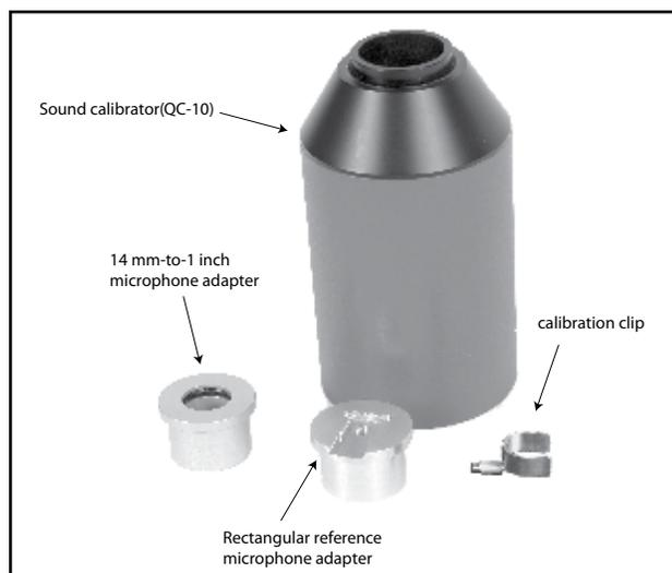
Figure C-4: Microphone calibration equipment
