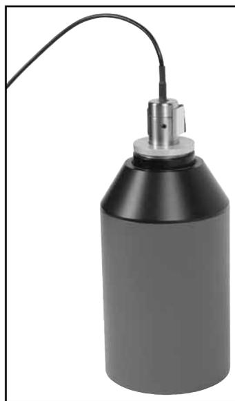
Figure C-1: Coupler microphone inserted into sound calibrator.
