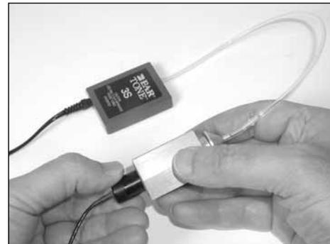
Figure C-8—Coupler microphone inserted into HA-2 coupler
