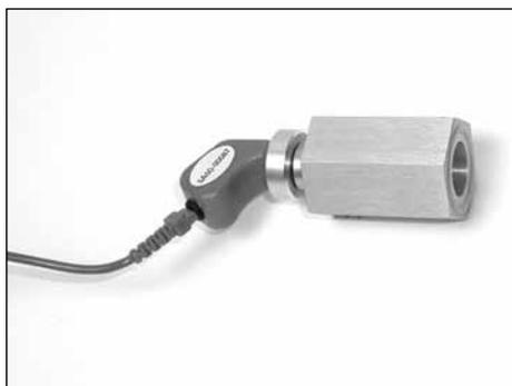
Figure C-9—Insert earphone connected to earphone calibration adapter and coupler
