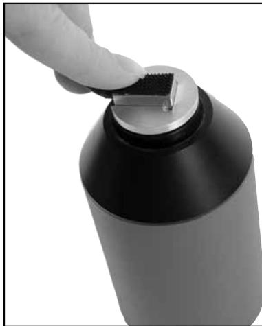
*Figure C-5A: Rectangular reference microphone inserted into sound calibrator*
