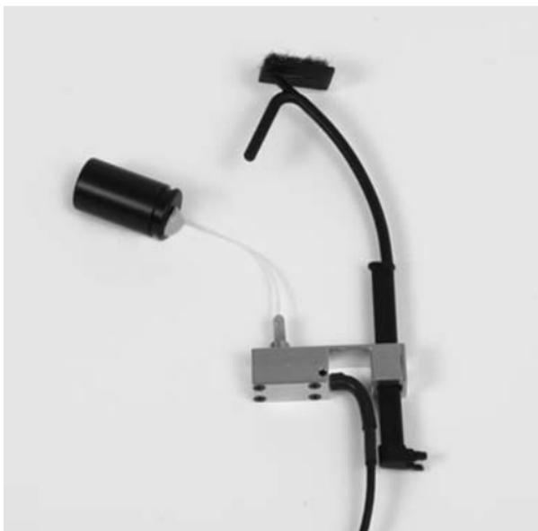
*Figure 4: Probe tube inserted through probe microphone adapter.*
