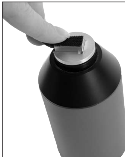
Figure 2: Rectangular reference microphone inserted into sound calibrator.
