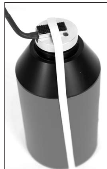
Figure 3: Using a rubber band to hold the microphone in place on the calibrator.
