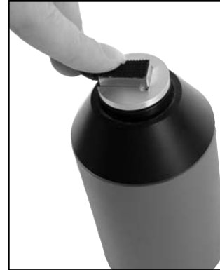
Figure 5.1.3: Rectangular reference microphone inserted into sound calibrator.
