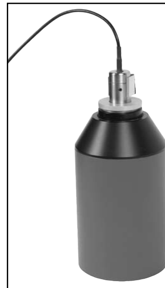
Figure 5.1.1: Coupler microphone inserted into sound calibrator.
