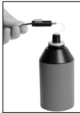
Figure 5.1.2B: Old-style probe microphone inserted into sound calibrator.
