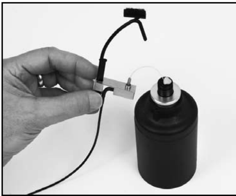
Figure 5.1.2A: Integrated probe microphone inserted into sound calibrator.
