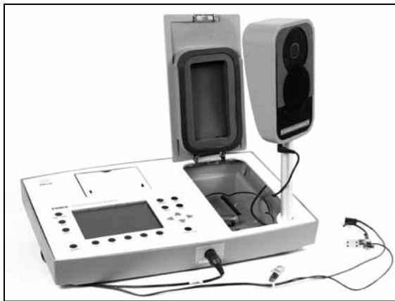
Figure 4.2.2—Internal sound field speaker setup
