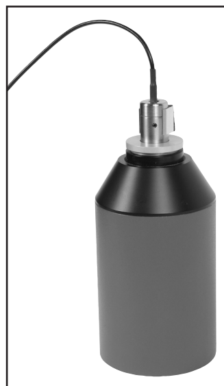
Figure C-2: Coupler microphone inserted into sound calibrator.
