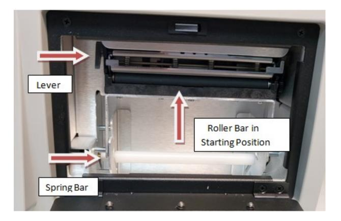
6. Load paper roll so it come off the back of the spindle and drop into the slots on either side of the white bottom spring bar
