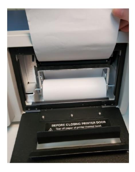
8. Feed Paper though door slot, close printer door and tear off extra paper.
