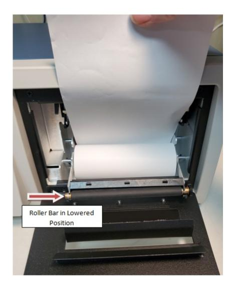
7. Move roller Bar back up and push until it clicks back in to starting position with paper behind it.
