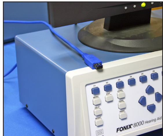
Figure 3: Place the wireless dongle in clear sight
