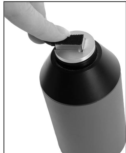
Figure C-4: Rectangular reference microphone inserted into sound calibrator.
