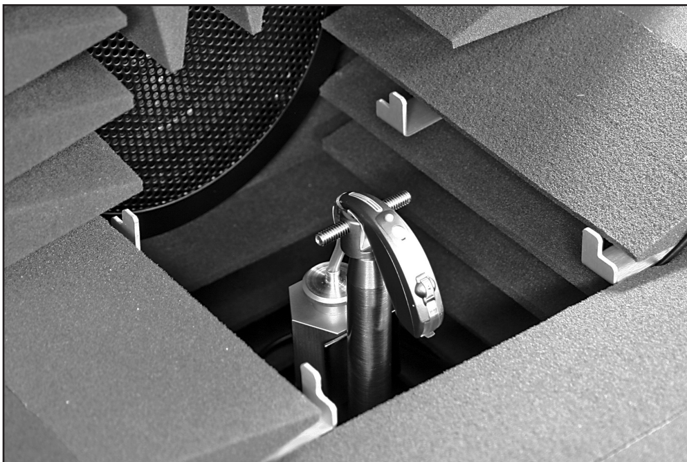
Figure 6.3.1D: Setting up a BTE hearing aid in the 8120 Polar Plot Chamber
