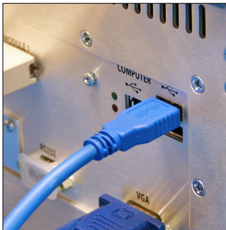
Figure 2: Plug USB cable into 8000
