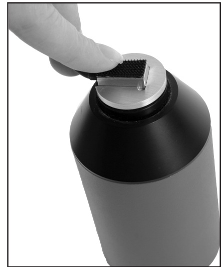
Figure C-4: Rectangular reference microphone inserted into sound calibrator.
