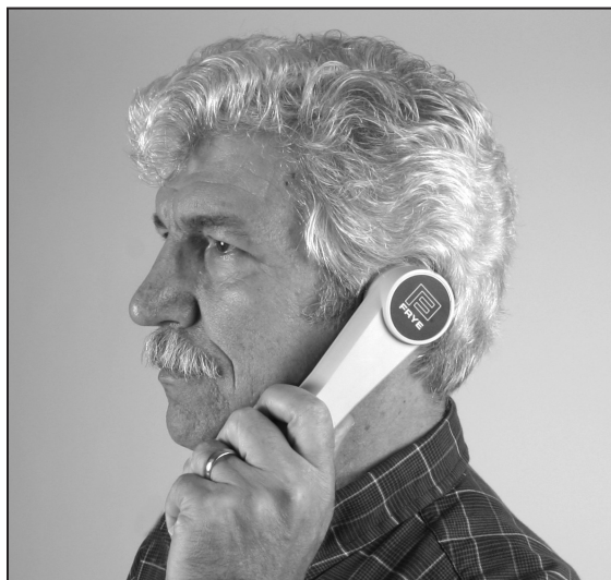
Figure 5.7.6A—Measuring telecoil response with the Telewand.
