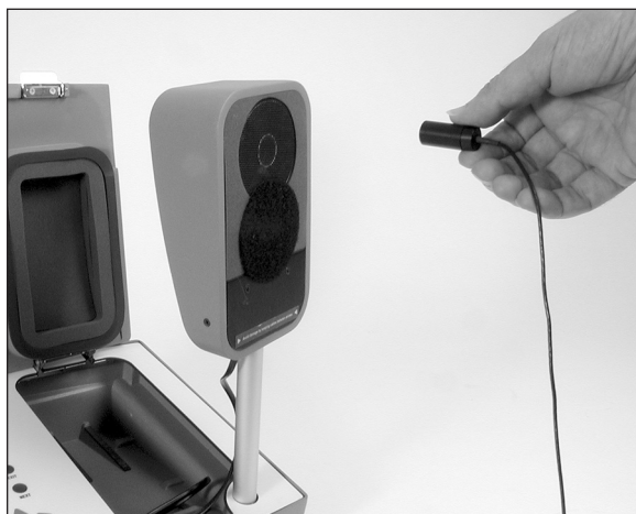
Figure 3.8.2B—Hold microphone six inches from the speaker
