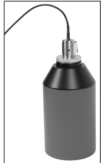
Figure C-1: Coupler microphone inserted into sound calibrator.
