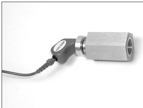
Figure C-9—Insert earphone connected to earphone calibration adapter and coupler
