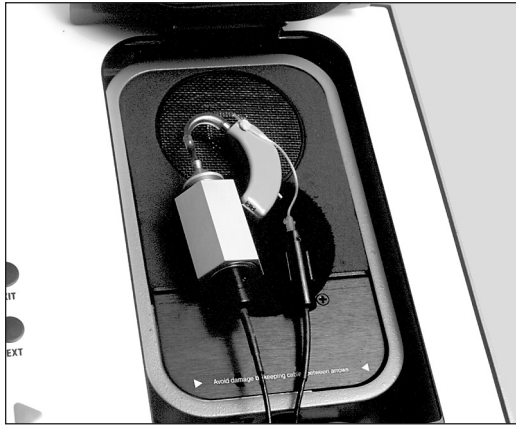
Figure 3.8.3—Leveling and testing using the reference microphone
