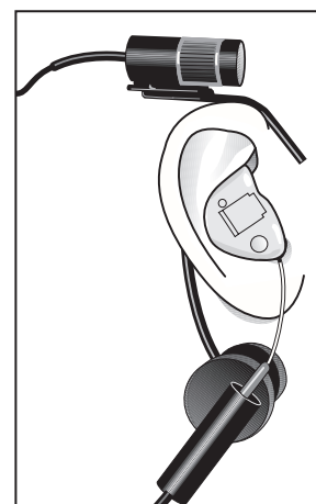
Figure 5.2.4D Real-ear setup using M300 separate microphone set.
