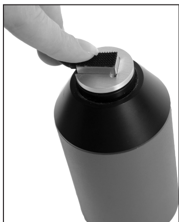
Figure C-5A: Rectangular reference microphone inserted into sound calibrator
