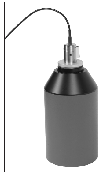
Figure C-2: Coupler microphone inserted into sound calibrator.
