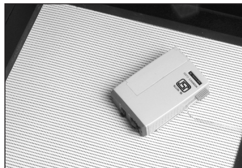
Figure 3.3.5B—Body Aid in test chamber
